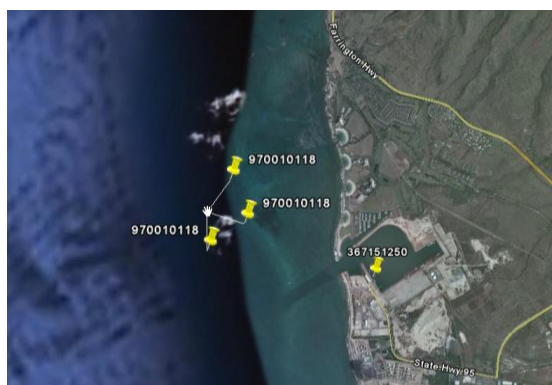
Figure 5: Zooming in shows 3 bursts detected from the AIS-SART at the deployed location 1.8 km, or ~1 nm, off the coast of Hawaii (test unit MMSI 970010118)
