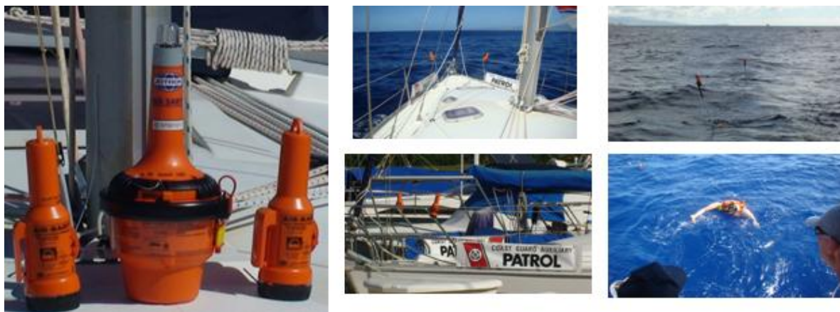
Figure 2: The AIS Test Units were deployed in various configurations in water and on deck
