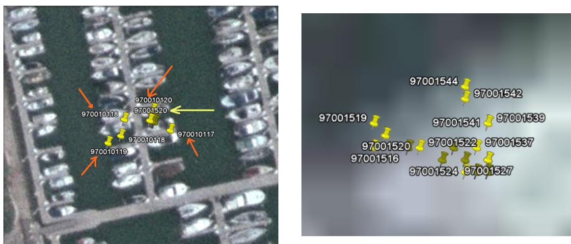
Figure 6: On Day 2 (left picture), several AIS transmissions were received from the AIS-EPIRB (...117), the AIS-SARTs (...118, 119 & 120) and the Class-A (...1520...) and zoomed in (right picture) shows the multiple incrementing numbers from the Class-A unit on the vessel
